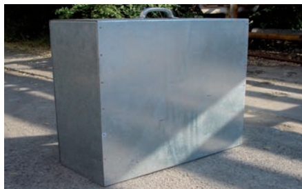
Sound insulation hood for the power unit
